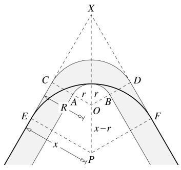
Note  $\angle PEX = \angle OCX = 90^\circ$  because they are tangents. Note POX is the line of symmetry so bisects the angles at O and P. Note  $\angle COX = 60^\circ$  because the arcs are a third of a circle and  $\angle EPX = 60^\circ$  because PE and OC are both perpendicular to the tangent EX, so they are parallel.
